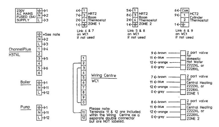
Note: - The ChannelPlus H37XL Programmer does not require an Earth connection. Therefore if mains Earth is connected to terminal 1 on the WC1 wiring centre, the Earth terminal on the H37XL backplate does not need to be connected.
